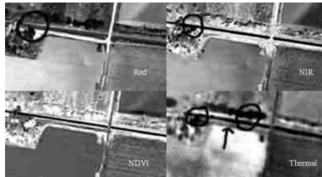
Figure 6. Airborne multispectral images of a concrete canal section in the Delta Lake Irrigation District (Case 2). The circled areas in the images show dense vegetation and surrounding areas, which was proven to be a tree and its shadow. NDVI with NIR and red images could differentiate the tree and shadow, but the thermal image could not
